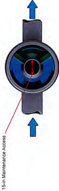
Fig.3 The central opening to the sump of the First Defense®-HC is 15 inches in diameter.
